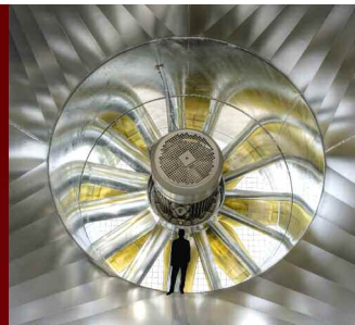
Axial fan with air flow volume up to 150 000 m 3 /h and upstream guide vane. Application: Realistic simulation of different air flow situations.
