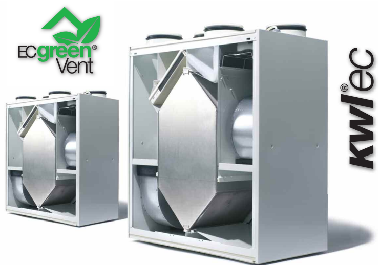
Compact wall unit with EC technology and heat recovery. Air flow rates 200 till 500 m³/h. Certified for passive house standard.
