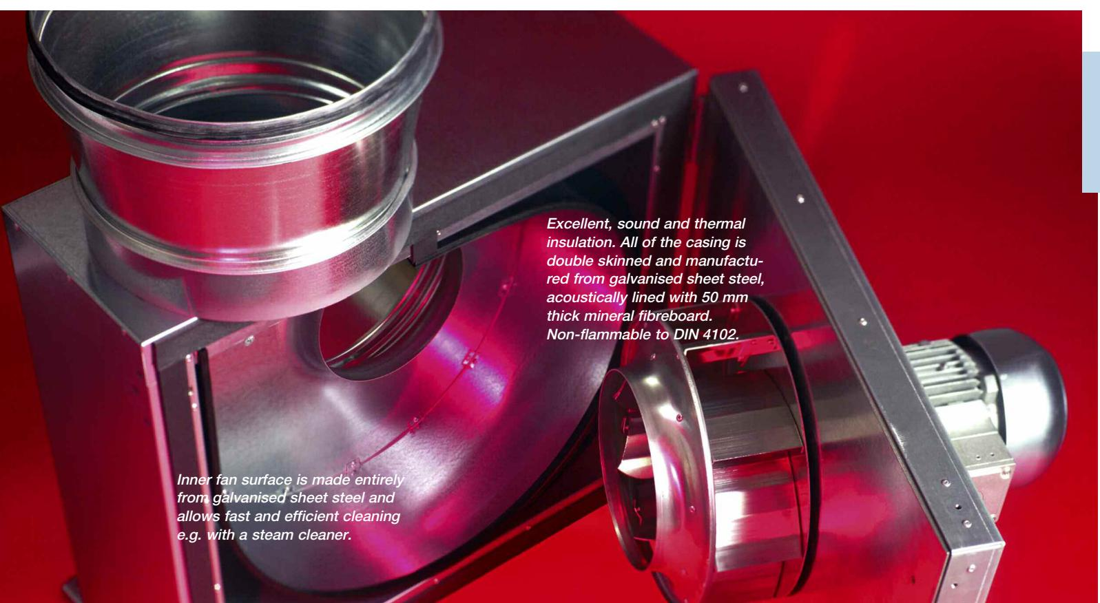
Inner fan surface is made entirely from galvanised sheet steel and allows fast and efficient cleaning e.g. with a steam cleaner.
