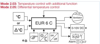
\* e.g. for EC-Motor, shutter, frequency inverter
