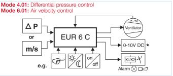
\* e.g. for EC-Motor, shutter, frequency inverter
