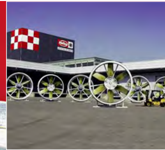
Axial fans of the type range AVD DL.. with an impeller diameter 3 150 mm. Complete output: approx. 3 Mio. m³/h. Use: In cooling towers of two paper mills.
